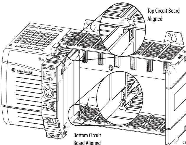
2. Slide the module into the chassis until it snaps into place.
