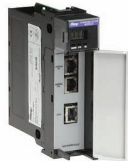
ESR2 Module: 112073-0001 1 Ethernet + 2 Serial Ports
